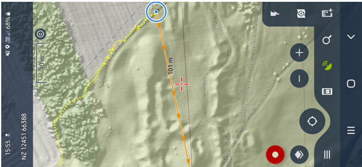
Practice navigation on my local golf course using a semi-transparent LIDAR (DSM) hillshade overlaid on, and providing a 3D view to the free Locus Map base. Current location shown by blue circle at end of a yellow bread-crum trail of the route I have followed. The orange line shows the direction the phone is pointing (west towards a set of three bunkers below a green) showing direction to follow. Controls at the bottom of the screen are optimally setup to provide easy access to features (e.g. to turn overlays on or off, add points of interest) that you may need in the field.
